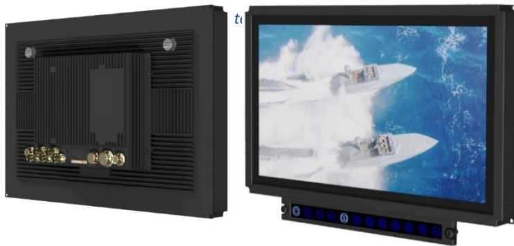
Figure 5 – LCD Module with DEU and UIM attached.
