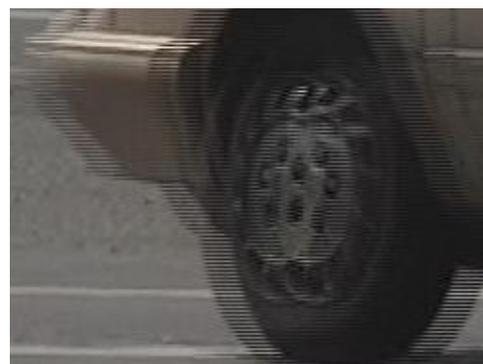
**Figure 7 - Field tearing in an interlaced image.**
